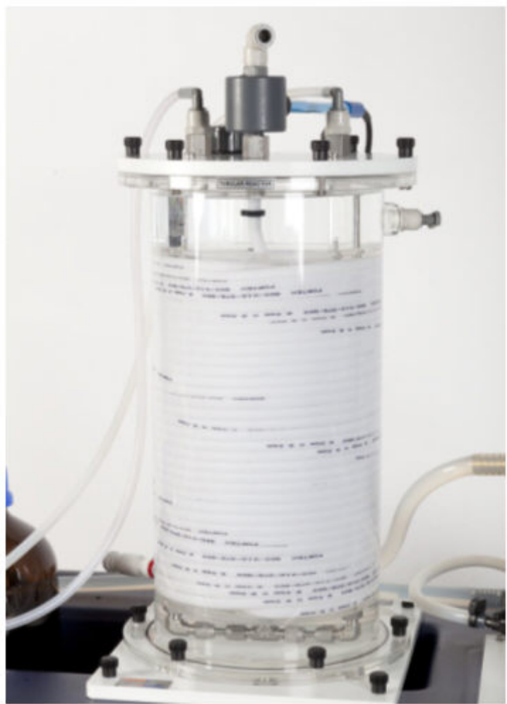
CEXC fitted with CET MkII tubular reactor
